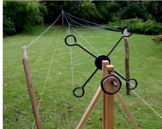
Figs. 1a, b: Left : a technical object – one geoglyph on the pampa. © Google Earth: geographic latitude \phi = 14^{\circ}33'22''\text{S} , longitude \lambda = 75^{\circ}10'40''\text{W} . Right : a functional model of a rope twister made from metal (in a convenient size) after the geoglyph on pampa (figure a), for experimental rope making. Original material might be hard wood. © J. Sonnek, 2013.
