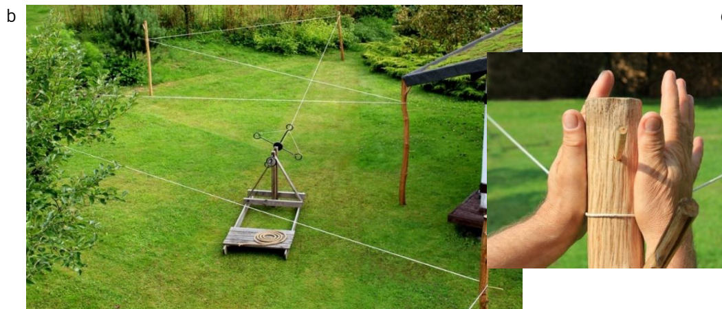
Figs. 2b, c: (b) One of Sonnek's experiments to make a long string, using a device inspired by the geoglyph discovered on pampa (shown in Fig. 1a); (c) the rope at the turning point; © J. Sonnek, 2013.
