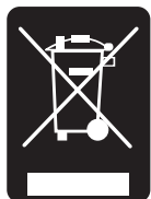
Fig. 1.4: Product labeling in accordance with EN 50419
